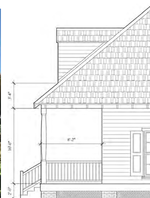
Typical Creole Style Broad Front Example and Massing Detail
