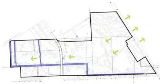
Figure A.3 Existing Drainage
