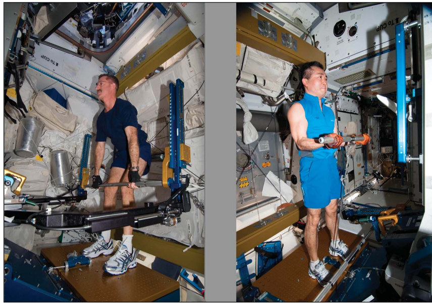
Images showing astronauts' demonstration of deadlifts and curls using the ARED 11
