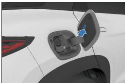
The charging warning label is attached on the inside the cover of the charge port.
