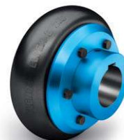
ELPEX-B elastic tire couplings Rated torque: 57 Nm ... 19,000 Nm
