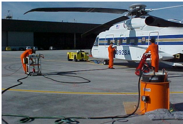
Thermosafe Induction drum heater, with a test Sikorsky S-92 aircraft being fuelled from a barrel of hot JP-8 fuel at 136°F
