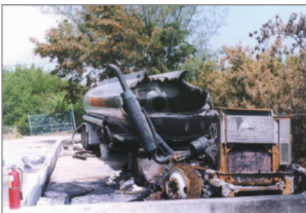
Fig. 2 – Top to bottom, Vehicle 1, 2 and 3. The NTSB concluded that the damage and fire on the other two vehicles resulted from exposure to heat from the fire on Vehicle 1. Combined all vehicles contained approximately 9,200 gallons of fuel that would have fuelled the blaze.
