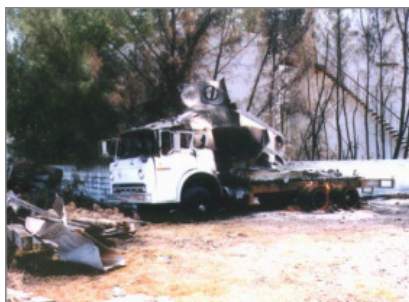
Fig. 2 – Top to bottom, Vehicle 1, 2 and 3. The NTSB concluded that the damage and fire on the other two vehicles resulted from exposure to heat from the fire on Vehicle 1. Combined all vehicles contained approximately 9,200 gallons of fuel that would have fuelled the blaze.
