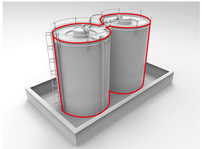
Fig. 1 – Storage tanks within close proximity of each other, means fires can viciously propagate through a tank farm if an incident is to occur.
