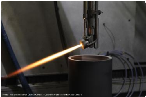
Mini-Nova HVOF over a cylinder bore. Photo: National Research Council Canada.
