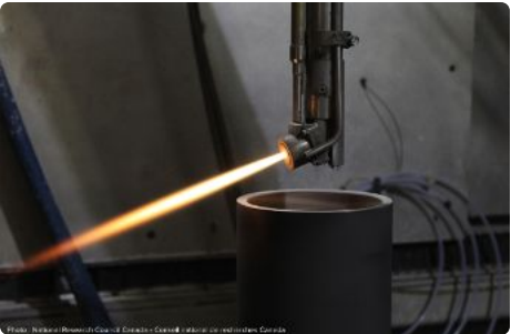
Mini-Nova HVOF over a cylinder bore. Photo: National Research Council Canada.
