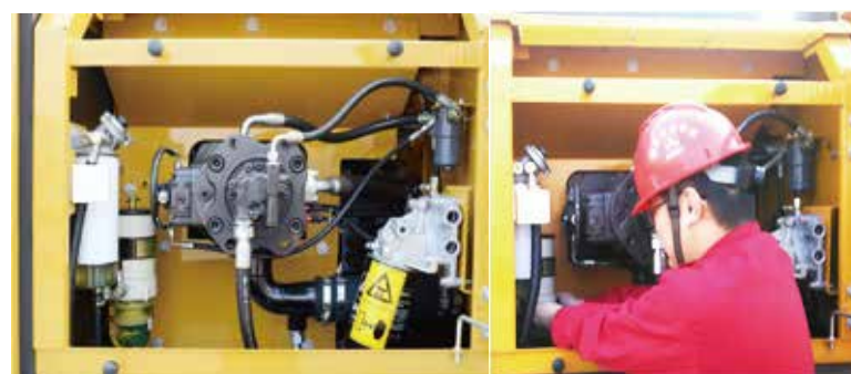
Replace diesel oil filter element
