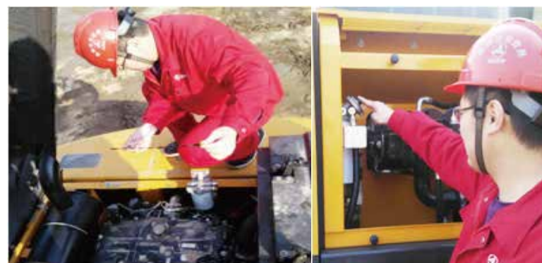
Inspect the situation of engine oil
