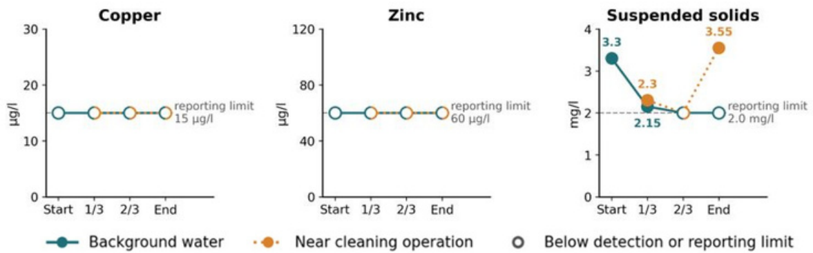
Fig.2: In-Situ water quality test results: Proactive grooming of an SPC coating
